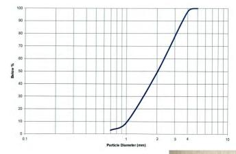
If the **Dionyssos "rice" marble fine gravel** is used in plastering, instead of the marble powder, the plastered wall surface gets a coarse, three-dimensional decorative effect, with pure white color, and with enhanced durability...
