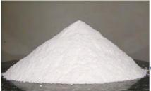
Bulk density: 1600 kg /m<sup>3</sup> Water absorption: 0.6%, Fines quality: SE > 70 MB <0.5 g/kg Water soluble material:<0.03%
