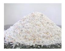
Bulk density: 1450 kg /m<sup>3</sup> Water absorption: 0.8% Fines quality: SE > 70, MB <0.5 g/kg Water soluble material: <0.03%
